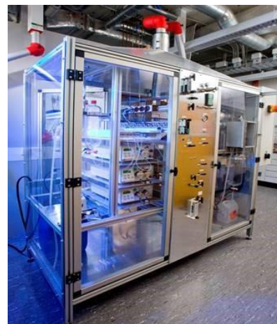
ECN.TNO lab-scale test facility (TRL3) for sorption-enhanced DME synthesis.
