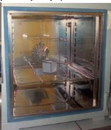
Isothermal oven test
