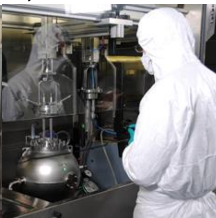
20-liters sphere apparatus for explosibility characterization
