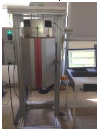
DTA/ATG for pre-screening of self heating of solids
