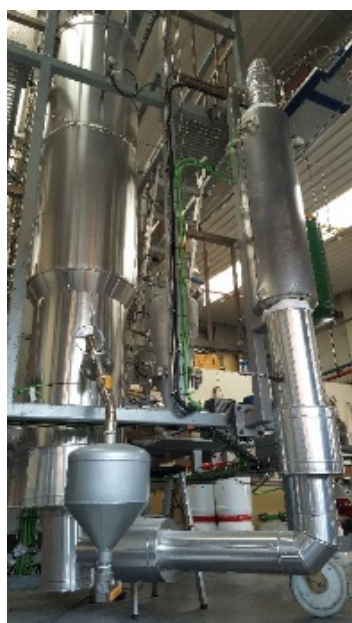
30 kW th bubbling fluidised bed facility at ICB-CSIC.
