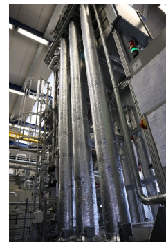
Six-column SEDMES setup at TNO, 6 meter reactors each with 6 kg of bed materials
