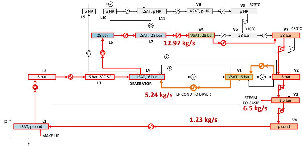
HRSC Power Output (target) = 7.0 MW
