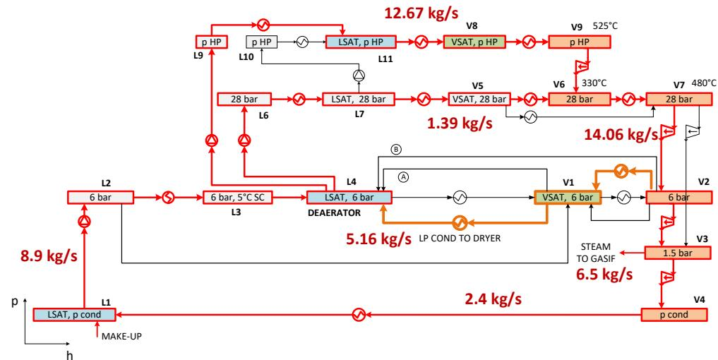
HRSC Power Output (target) = 12.4 MW
