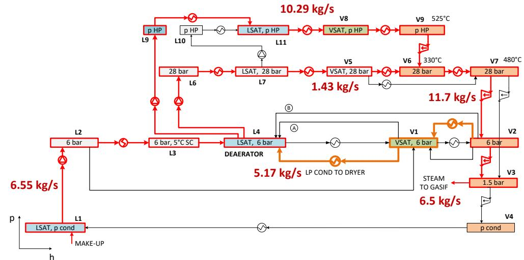
HRSG Power Output (target) = 9.2 MW
