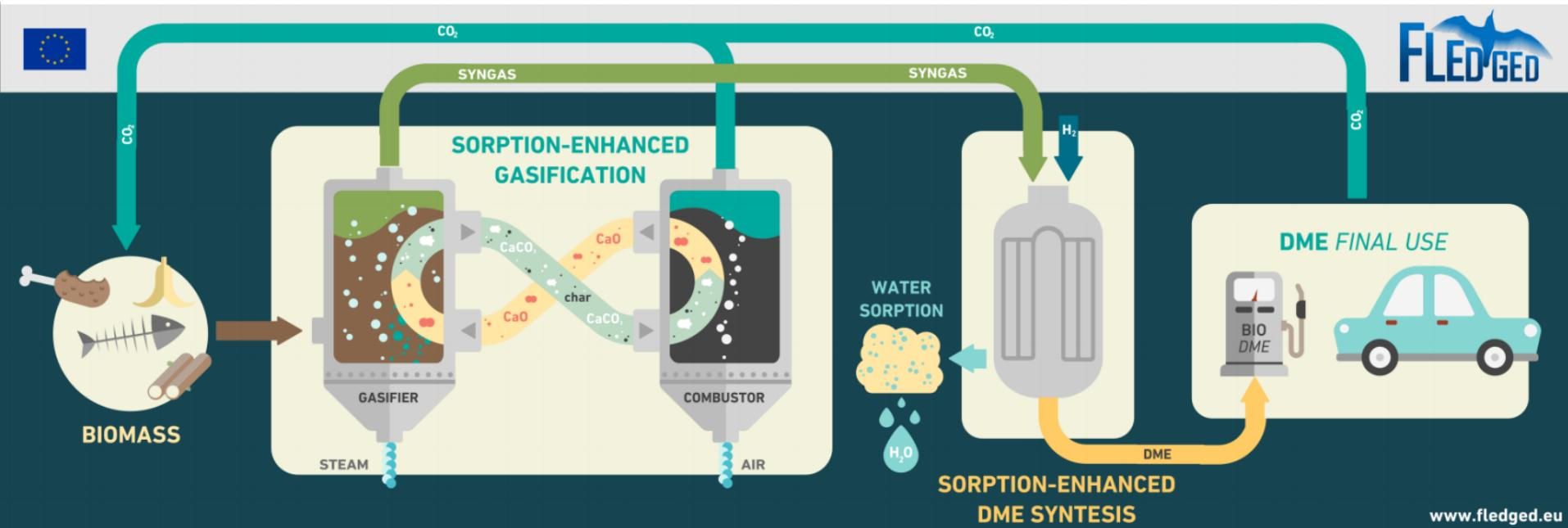
A novel highly intensified and flexible process for the **co-production** of **bio-DME** and **electricity** from biomass, coupling the indirect gasification with *in-situ* CO<sub>2</sub> separation
