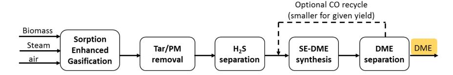
OBJECTIVE of this WORK: Solve the mass and energy balances of two synthetic fuel production plants based on sorption enhanced gasification, one focused on DME and other on Synthetic Natural gas (SNG), to compare their performance
