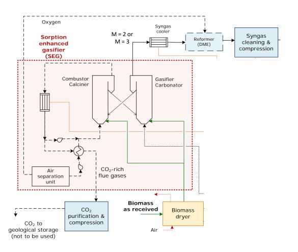
Objective: M-module=2 (DME) and 3 (SNG) after the cleaning and compression
