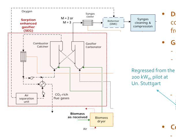
**Drying**: tube bundle dried using condensing steam at 6 bar. Moisture from 45 to 20%wt.
