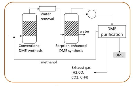
Two sequential reactors: conventional direct DME + SE-DME
