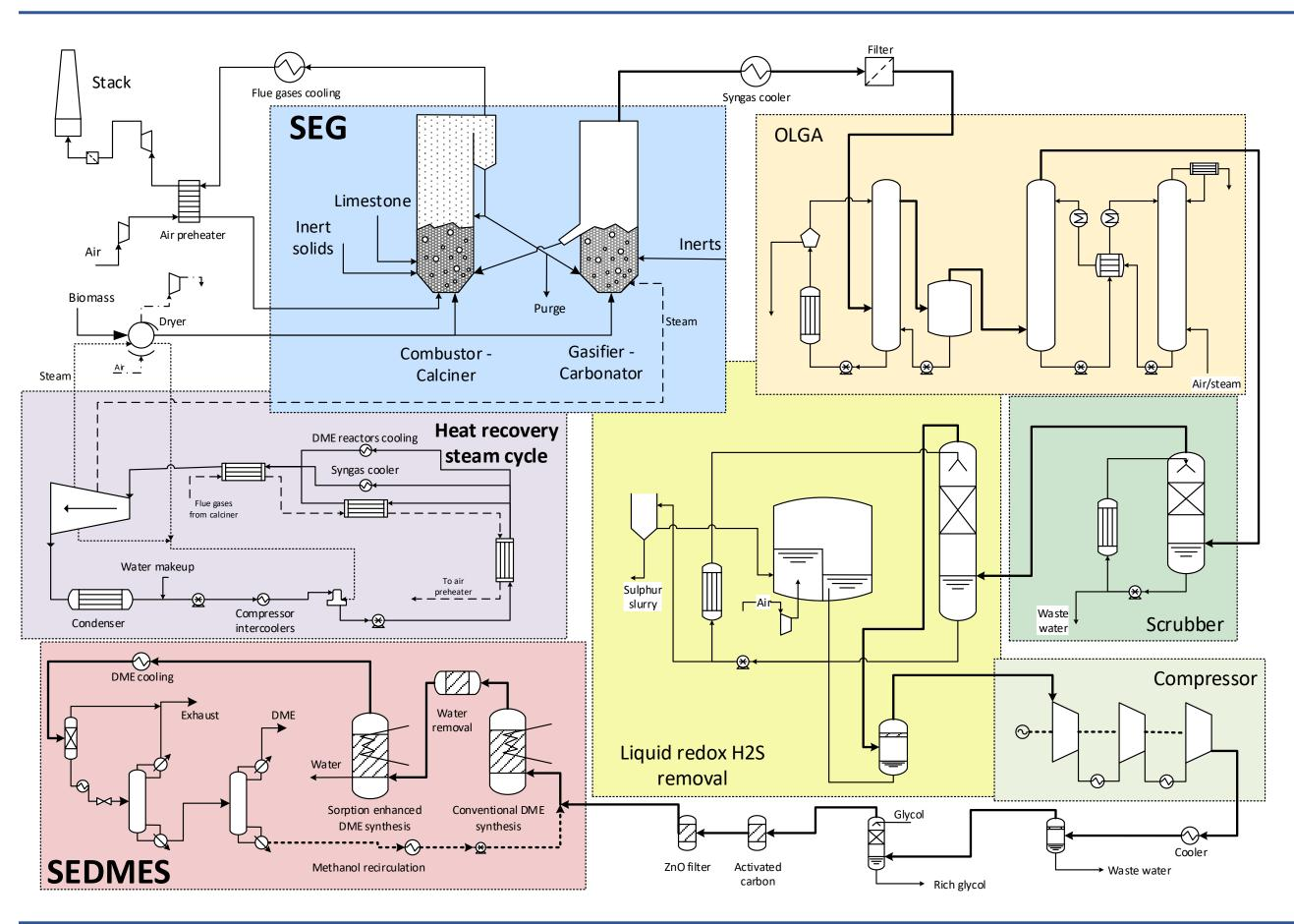
The process combines flexible **sorption enhanced gasification** (SEG) and **sorption enhanced DME synthesis** (SEDMES) technologies to produce DME from biomass. SEG:
