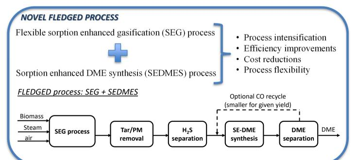
Flexible SEG process will be demonstrated at TRL5 in the 200 kW dual fluidized bed facility at University of Stuttgart.
