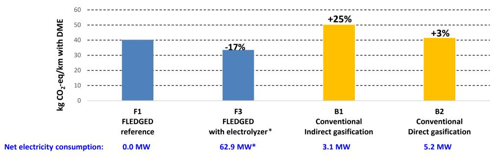
The parameters influencing the environmental impact (carbon footprint) are the process yield (kg of DME produced with a given biomass input) and the net electricity consumption.
