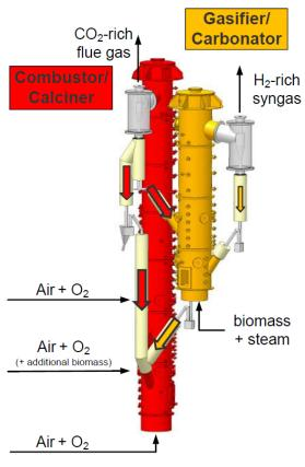
200 kW<sub>th</sub> dual fluidized bed facility at University of Stuttgart
