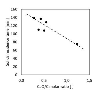
Increasing the amount of calcined CaO into the gasifier (CaO/C) makes  $\tau$  to be reduced
