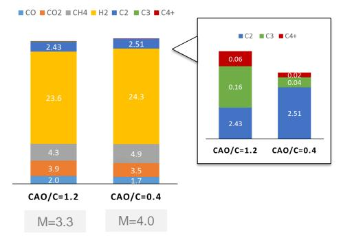
Slightly higher  $H_2$  contents as  $\tau$  is increased (lower CaO/C) and so M-modules
