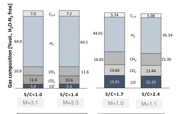
✓ No significant influence on permanent gases (M-module constant) and light hydrocarbons content.
