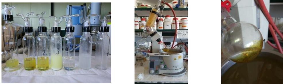
Figure 7 Example picture of impingers after tar sampling (left) and rotary evaporator (middle) used to concentrate samples and determine gravimetric tar (right)
