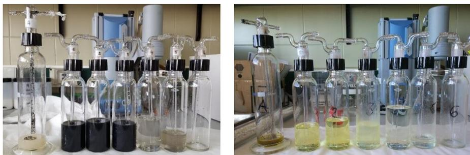
**Figure 15 Pictures of the tar sampling impingers for the SEG experiments with wood pellets at (left) S/C=1.4, CaO/C=0.30 and 717 °C and (right) S/C=1.6, CaO/C=0.36 and 665 °C**
