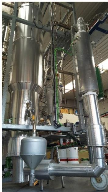
Figure 1 Picture of the 30 kW<sub>th</sub> BFB gasifier at ICB-CSIC
