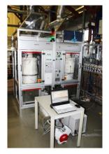
At ECN, several steam sorbents have been screened in the socalled "Spider" facility. This high-throughput rig allows assessing the performance of mixtures of commercial catalyst and sorbents under SEDMES conditions. Based on a literature review, a list of water sorbents candidates has been drafted.
