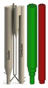
Accurate models are needed to support development and scale-up of new processes, such as sorption enhanced gasification (SEG). At LUT, the development of a modelling tool for comprehensive simulation of interconnected CFB reactors for indirect gasification is ongoing. In particular, a three-dimensional semi-empirical model is available, which can be applied to air/oxygen-fired combustion, gasification and calcium looping.
