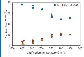
Optimal conditions for downstream DME production are reached at a gasifier temperature of about 715 °C.
